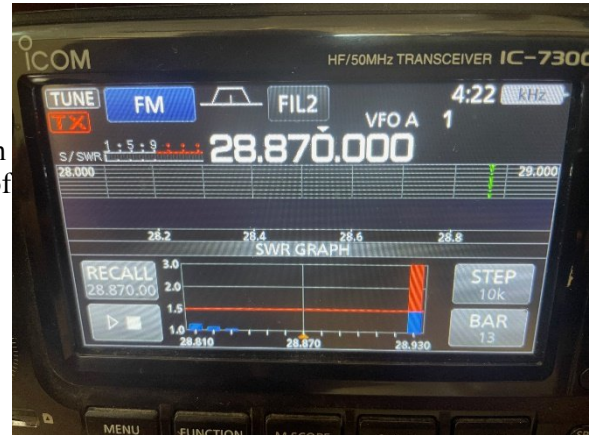
Fig. 3. Tuned 10-m is flat
