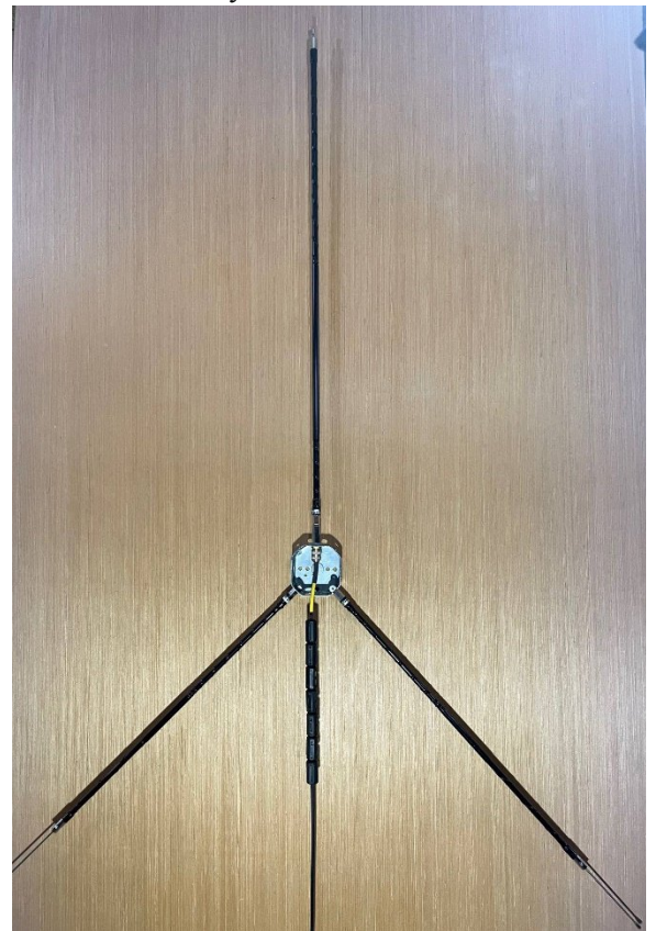
Fig. 1. Triad antenna, 40-m radiator
