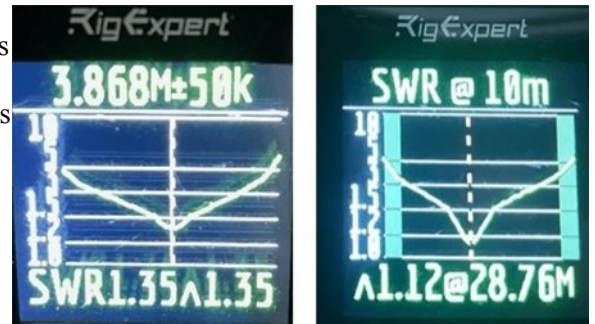
Fig. 2. Measured SWR, left 80-m, right 10-m
